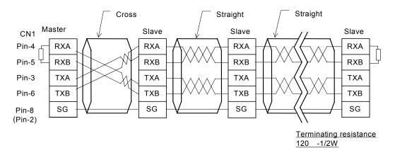
\* When using 2-wire type, short RXB to TXB and RXA to TXA.
